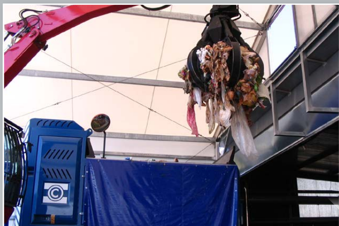
Caricamento FORSU con polipo Loading of HSOF with orange peel grab
